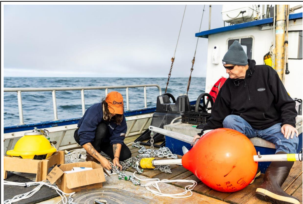
Fully assemble the mooring on deck. The Spotter, the Polyform float/marker and the anchor are all shown here. Double-check all connections.
