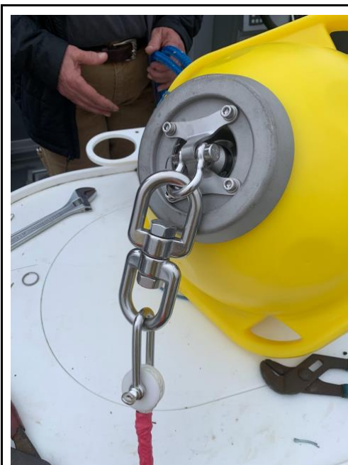
Fully assemble the mooring on deck. The Spotter, the Polyform float/marker and the anchor are all shown here. Double-check all connections.
